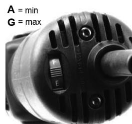
Fig. 6: Speed adjustment
