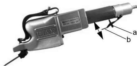
Fig. 3: Freeing the lever valve DL 40
