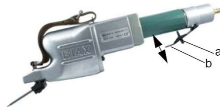
Fig. 3: Freeing the lever valve DL-40
